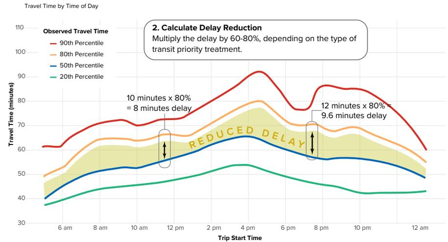
Figure 2-7 How to Calculate Potential Delay Reduction per Treatment – Step 3
