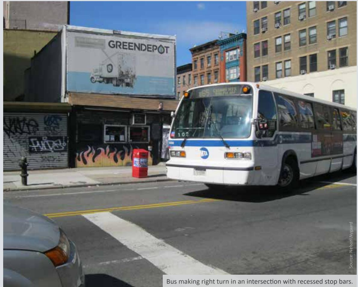
Bus making right turn in an intersection with recessed stop bars.
