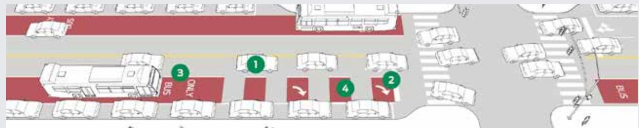
Transit Approach Lane (top) and Queue Bypass (bottom); green numbers highlight pavement marking features.
