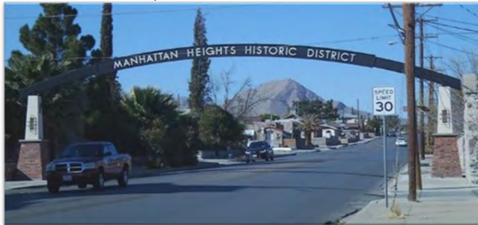
Sample Vertical Clearance Monument (Archway)
