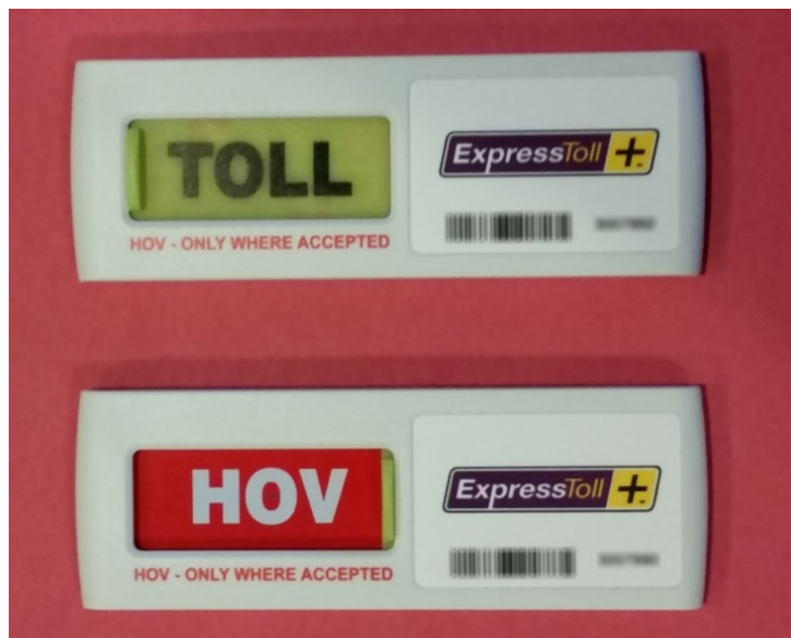
Figure 5-12: ISO 18000 6c Switchable Transponders with Color Coded Status Indication
